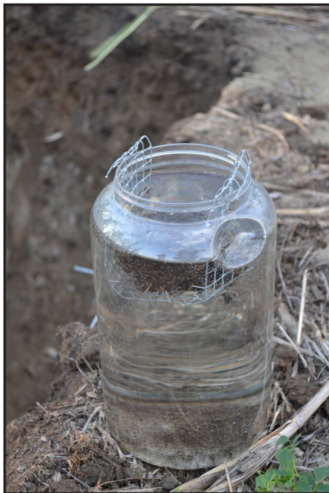
“Slaking” tests involving clumps of soil and jars of water help farmers see firsthand the benefits of building healthy, stable soil. (LSP photo)
